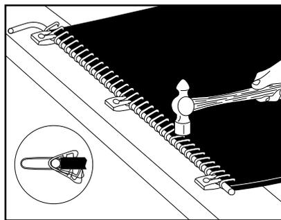
5. Turn belt over and hammer lacing halfway into bottom of belt.
