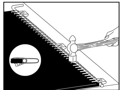
6. Hammer lacing completely into top of belt.
