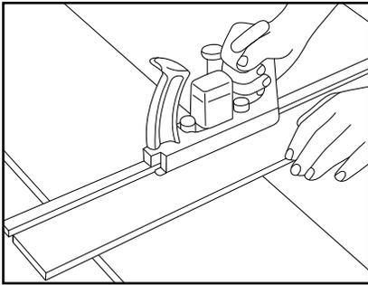
1. Square belt ends, then cut using the Alligator® 300 Series belt cutter.
