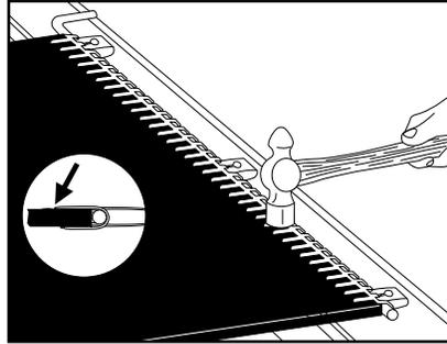
8. On hard steel plate, hammer again from top, until teeth are flush with belt surface.
