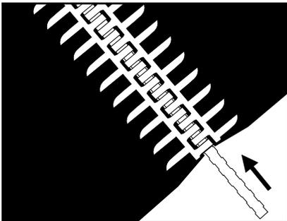
10. Repeat steps 1 thru 9 for other end of belt, insert hinge pin and notch belt.
