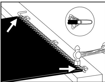
4. Using a soft wood surface for support, hammer end teeth halfway into top of belt.
