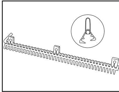
2. Place clips on lacing and insert gauge pin.
