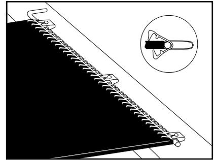
3. With bar side up, center lacing on belt holding belt against gauge pin.
